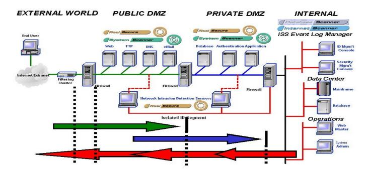
RealSecure is a network and host based intrusion detection and response. RealSecure Sensors are composed of network sensors that are installed on the network on critical sub-networks and host sensors that are installed on critical production servers. A RealSecure Management Console centrally manages all sensors. Communication between the console and sensors is originated at the console and is strongly encrypted and authenticated using a public/private key authentication mechanism.
